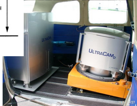
Figure 6 Conventional Photogrammetry Aerial Cameras (Top to Bottom) – RC30 Film Camera, UltraCamD Digital Camera Source: New Tech Services Inc.
