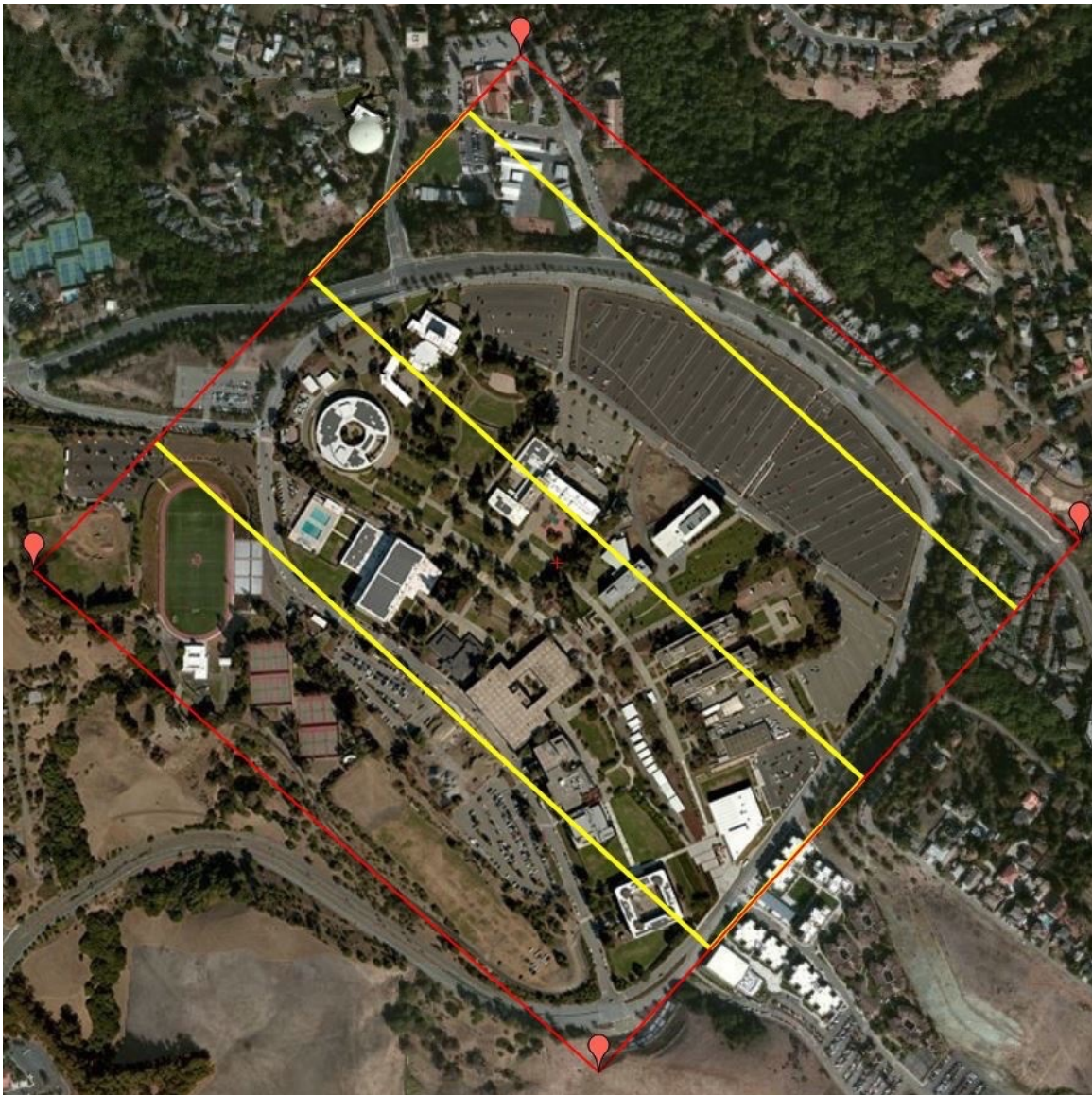
Figure 12 Conventional Photogrammetry Mapping Mission Flight Plan Red Polygon Represents Area of Interest, Yellow Lines Represent Flightlines Example: 3 Flightlines, 18 Photos (179 acres, CSUEB Campus)
